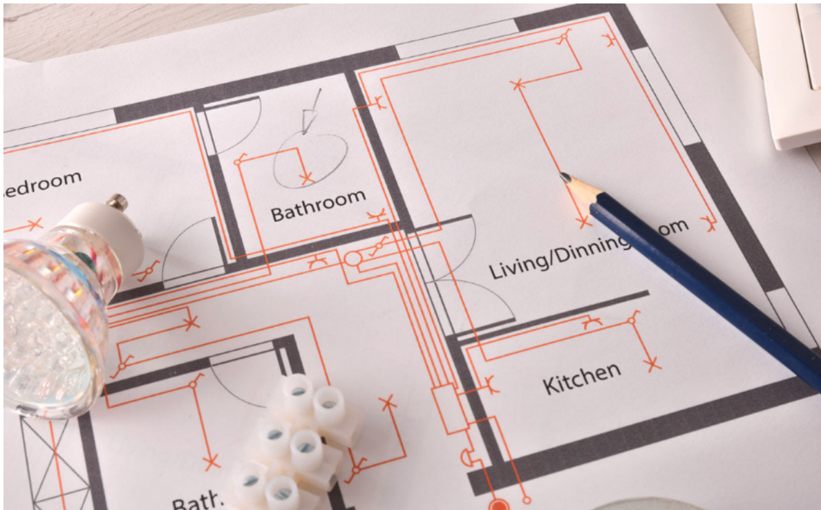
Fig. 5.1.62 Electrical installations plan
