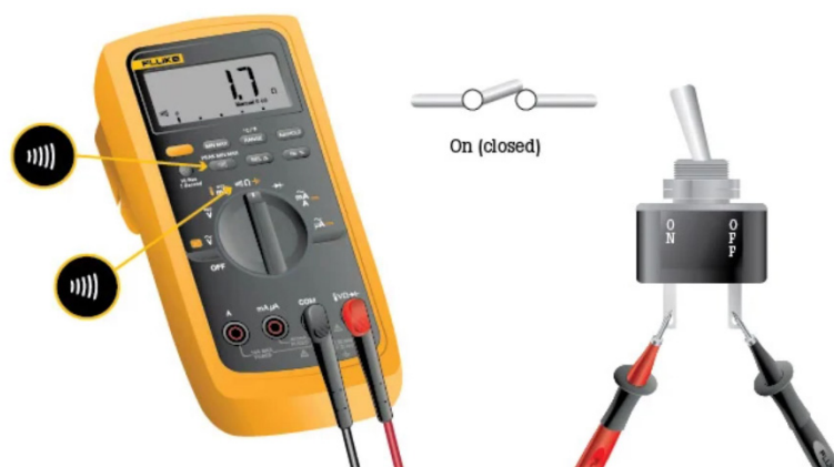
Fig. 5.3.18 Testing the connection
