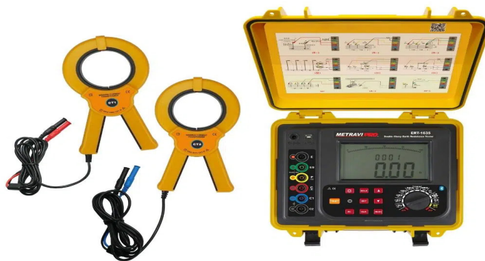
Fig. 3.3.17 Grounding resistance measurement
