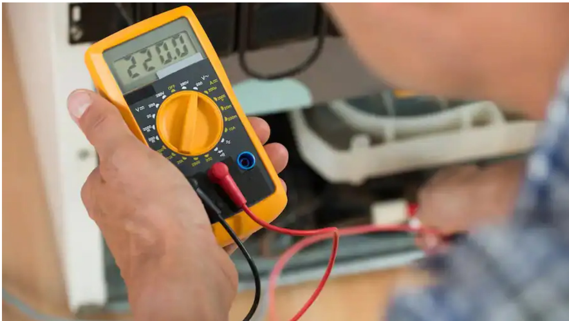
Fig. 3.3.33 Multimeter for voltage testing
