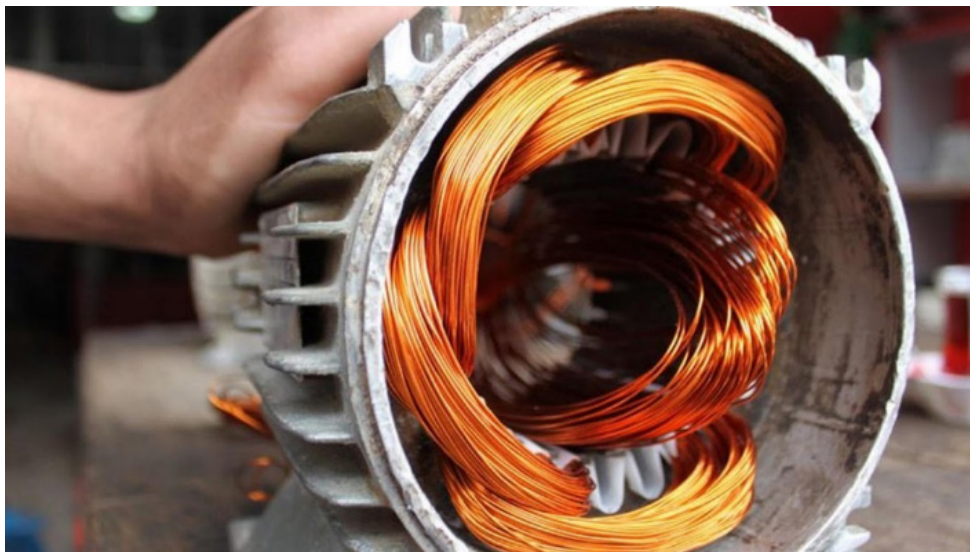
Fig. 4.2.22 Insulation between coils
