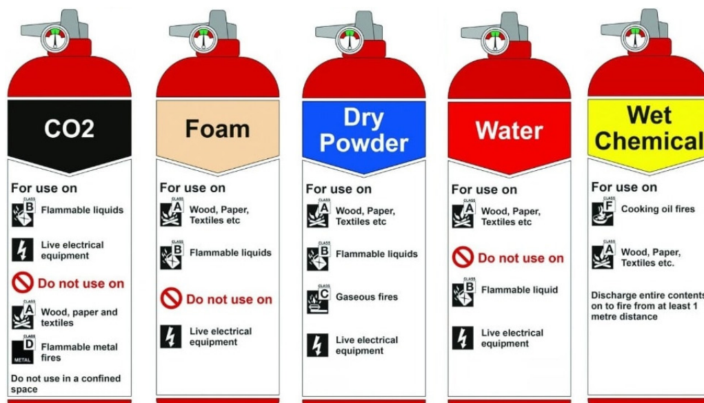
Fig. 8.2.4 Types of Fire Extinguishers
