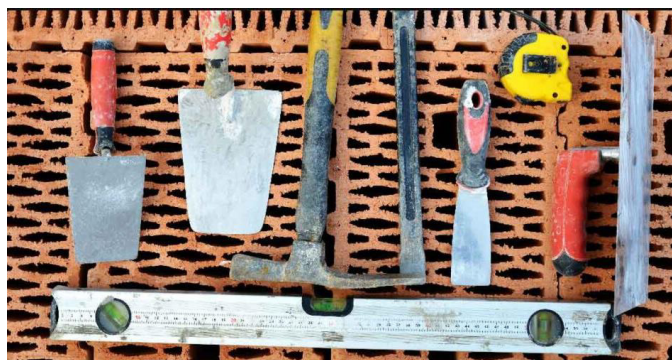
Fig. 4.1.4 Tools used for Block Work
