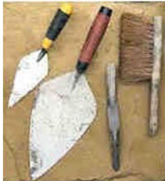
Fig. 3.7.2 Tools used in Pointing work
